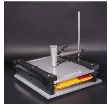
Fixture for ASTM F2054 restraining – restrains the package to ensure the pressure affects the package sealings in the correct way
