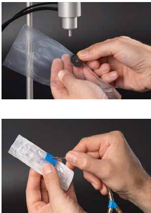
A septum ensures an airtight seal and protects the package from tearing. Different types of septa are suited to different packages and needles.
