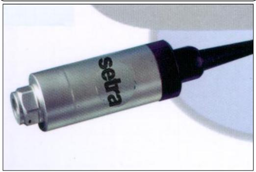
etra System's Model 567 high performance pressure transducer offers customer accessible downranging capabilities, making this unit ideal for high overpressure applications. The 5:1 turndown is easily accessed via a switch and potentiometer.
